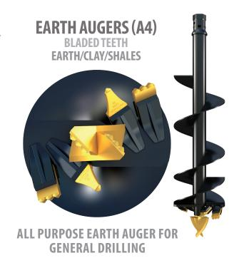
The angle and geometry of the teeth to the pilot is the key to the efficiency in which these augers perform. Available in earth or multi-faced tungsten (MFT) braised onto the face of the teeth, providing longer wear life and greater cutting performance. Not suited to harder fracturable rocks.
